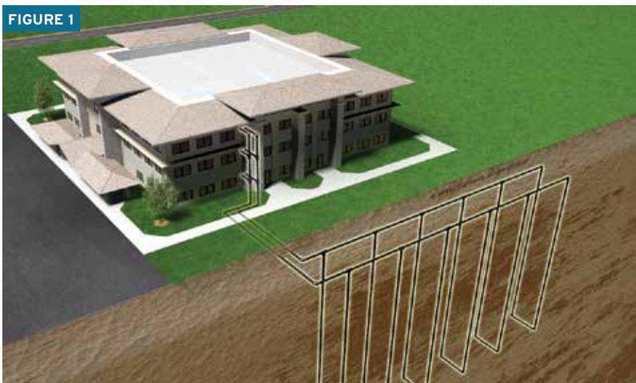
Figure 1: a commercial building with a vertical borehole ground heat exchanger.
